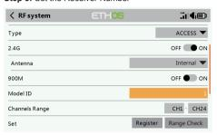
The system will assign you the receiver a number automatically, when you create a new model, and this can be easily changed. The range of the Model ID is 00-63, with the default number being 01. Once the receiver is set to the desired number and is bound to the TANDEM X20S, the bind procedure will not need to be repeated unless the receiver number is changed. At this point, set the receiving number to your preferred number and repeat the binding operation.
