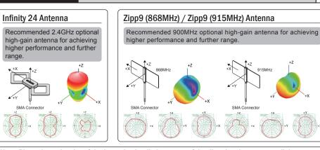
Note: Please keep the aircraft in the optimal radiation range of the directional antenna at all times
